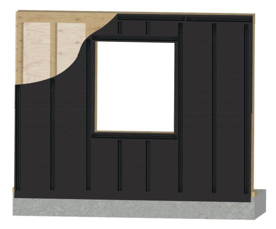
Apply vertical chalk lines every 16 inches on-center at the stud locations for Batten UV layout.
