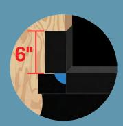
• To use HydorCorners instead of patches, place a HydroCorner in each sill corner and fasten in place with a staple. Install HydroFlash UV+ 9" to extend at least 6 inches up the inside of each jamb inside the window opening.
