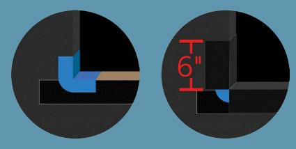
• To use HydorCorners instead of patches, set a HydroCorner in a bead of sealant at each corner sill and fasten with a staple. Install HydroFlash UV+ 9" to extend at least 6 inches up the inside of each jamb inside the window opening. HydroFlash has an acrylic adhesive that must be rolled in order to fully adhere to the substrate.
