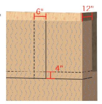
Flash wall penetrations (such as outlets, exhaust vents, etc.) with proper shingling technique to maintain drainage
