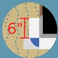
To use HydorCorners instead of patches, set a HydroCorner in a bead of sealant at each corner sill and fasten with a staple. Install
