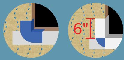
To use HydorCorners instead of patches, set a HydroCorner in a bead of sealant at each corner sill and fasten with a staple. Install
