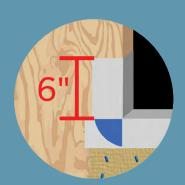
• To use HydorCorners instead of patches, place a HydroCorner in each sill corner and fasten in place with a staple. Install HydroFlash 9" to extend at least 6 inches up the inside of each jamb inside the window opening.
