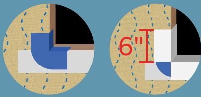
• To use HydorCorners instead of patches, set a HydroCorner in a bead of sealant at each corner sill and fasten with a staple. Install HydroFlash 9" to extend at least 6 inches up the inside of each jamb inside the window opening. HydroFlash has an acrylic adhesive that must be rolled in order to fully adhere to the substrate.
