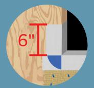
• To use HydorCorners instead of patches, place a HydroCorner in each sill corner and fasten in place with a staple. Install HydroFlash 9" to extend at least 6 inches up the inside of each jamb inside the window opening.
