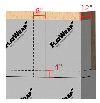
Do not let housewrap be exposed to sunlight in excess of 120 days prior to the installation of cladding
