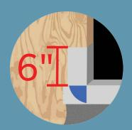
• To use HydorCorners instead of patches, set a HydroCorner in a bead of sealant at each corner sill and fasten with a staple. Install HydroFlash 9" to extend at least 6 inches up the inside of each jamb inside the window opening. HydroFlash has an acrylic adhesive that must be rolled in order to fully adhere to the substrate.
