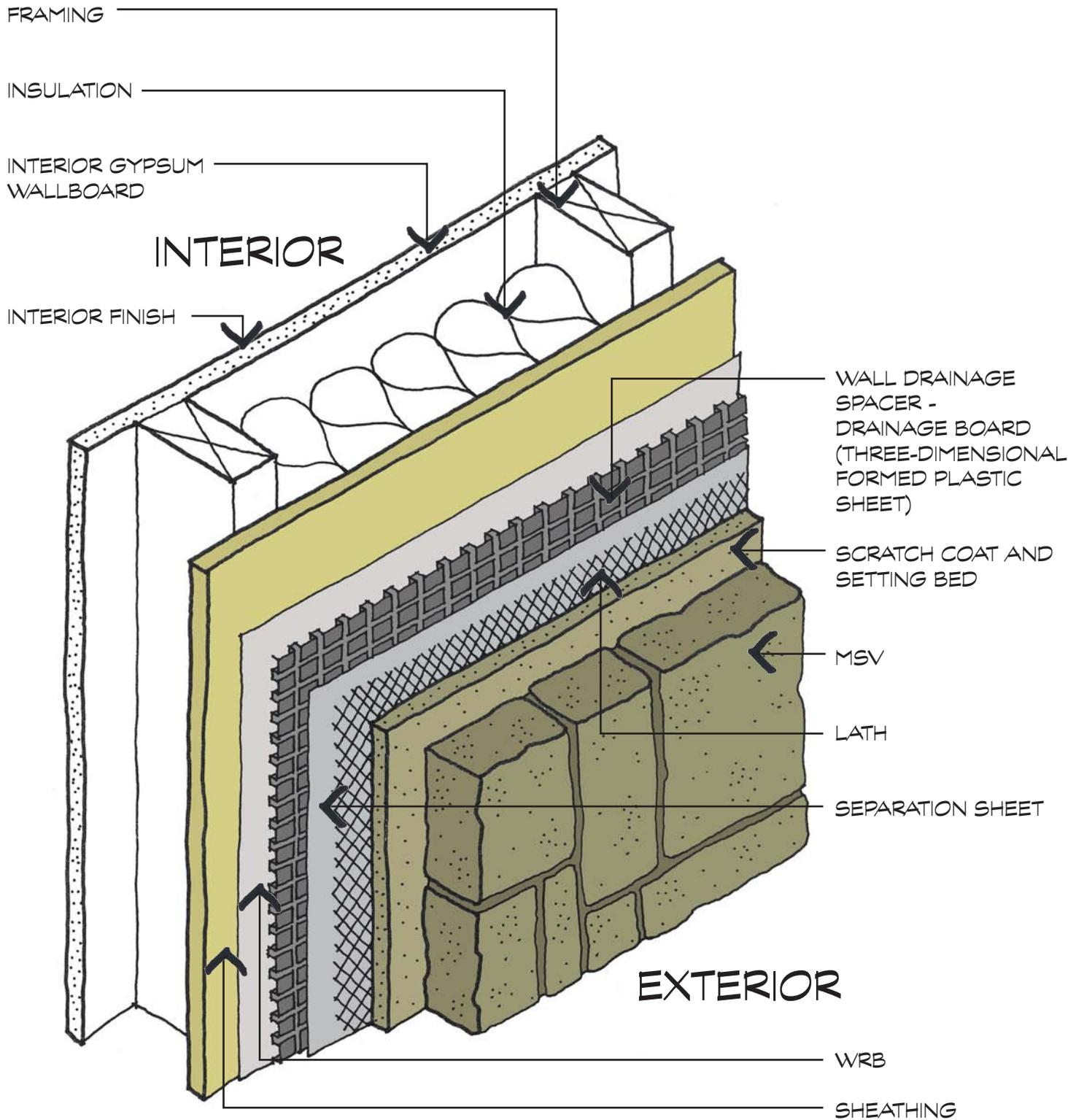
① ISOMETRIC OF WATER-MANAGED MSV ASSEMBLY
