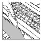
Step 4: Cut exposed excess felt away on shingles/shakes/ tiles. In areas of severe weather or rough hand split shakes, lay a bead of caulk between felt and Rapid Ridge 1/4 inch in from edge for entire length of Rapid Ridge.
