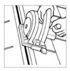
**Step 1:**Snap chalk line and cut slot 2 inches wide (1 inch on each side). Allow for a closed area of sheathing 12 inches at
