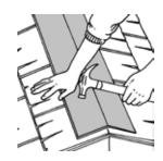
Step 5: Install 30 lb felt 7 inches wide on top of entire length of Rapid Ridge (optional on asphalt shingles).
