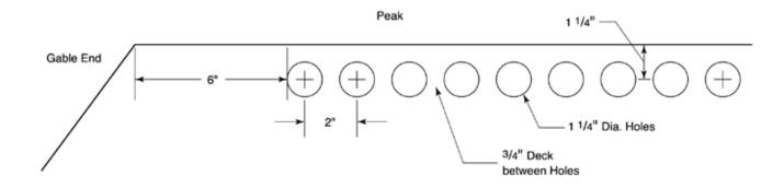
In certain areas of the United States, building codes do not allow for a continuous slot to be cut into the roof structure. This is especially true on the west coast and other earthquake-prone areas. Rapid Ridge can be installed on a roof without a continuous slot.
