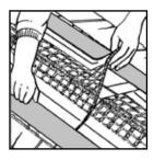
To splice, remove about 3 inches of matrix from fabric and lay end of new roll inside remaining fabric to create fabric overlap.
