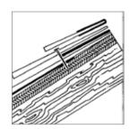
Step 2: Fold 30 lb. felt back over last course of shingles/ shakes/tiles exposing 2 inch slot. (When cutting last course of shingles/shakes/ tiles, use caution to avoid cutting through felt.)
